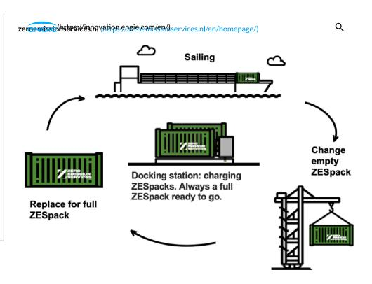
The charging stations can act as energy hubs that can stabilise the grid during peak loads and where other vehicles can also charge. Thanks to their mobility, ZESpacks can be used to supply and store energy at all kinds of locations, such as construction sites and festivals.
